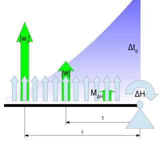
$\Delta H : \text{Angular momentum acceleration.}$   $\vec{r}: \text{Offset to point of contact.}$   $M_{\Delta H}: \text{Particle momentum.}$   $\vec{w} \& \vec{w_r}: \text{Angular velocity.}$   $\Delta s : \text{Collision contact stretch, relative to } M_{\Delta H}.$   $\Delta t_f: \text{Fixed time periodicy of simulation.}$   $\Delta t_d(\vec{r}): \text{Real contact duration time.}$  $c_{\Delta t} = \Delta t_d / \Delta t_f: \text{Regulating time coefficient.}$
